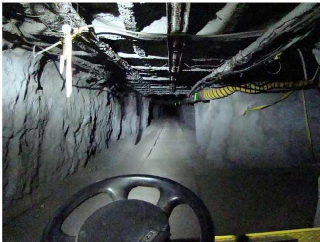
Fig. 2. Light distribution of the NIOSH LED cap lamp. The photograph was taken at the NIOSH Safety Research Coal Mine.
